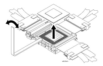
Note: The analysis probe cables should remain attached to the interposer throughout the installation/uninstallation process.
