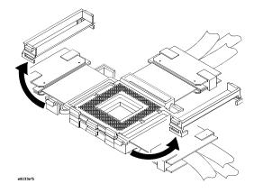
**3** Lift the heatsink from the processor.
