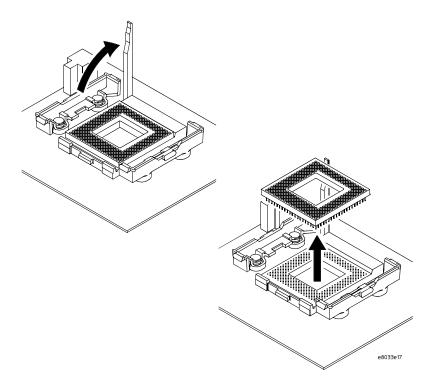
You can now install the microprocessor in the ZIF socket on the target system.
