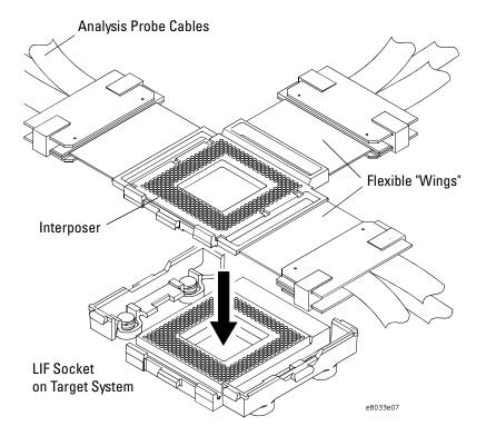
Note: The analysis probe cables should remain attached to the interposer throughout the installation process.
